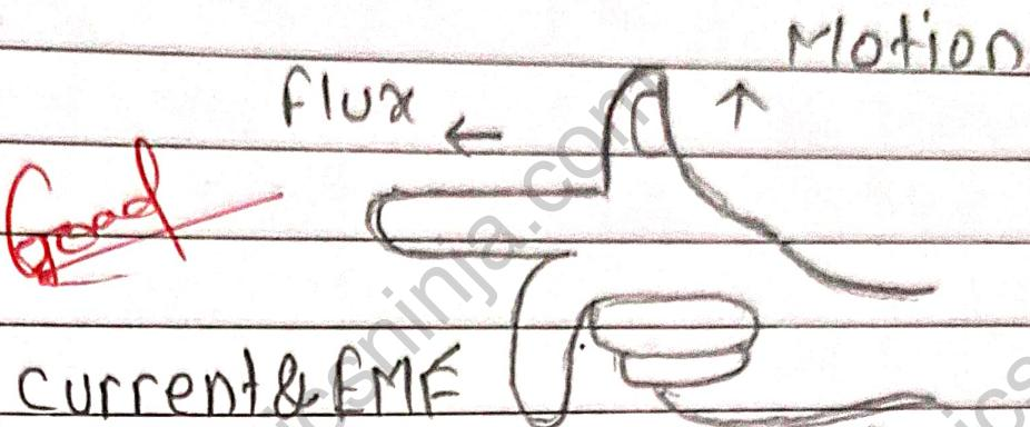
Let the thumb and first two fingers of the right hand be arranged in right angle with each other as shown in fig@
